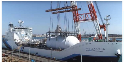
Cargo Tank Installation (7 March 2020) at KHI Harima Works
